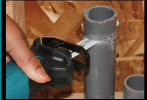
0 - 3,000 SPM combined with a 1/2" stroke for fast cutting
